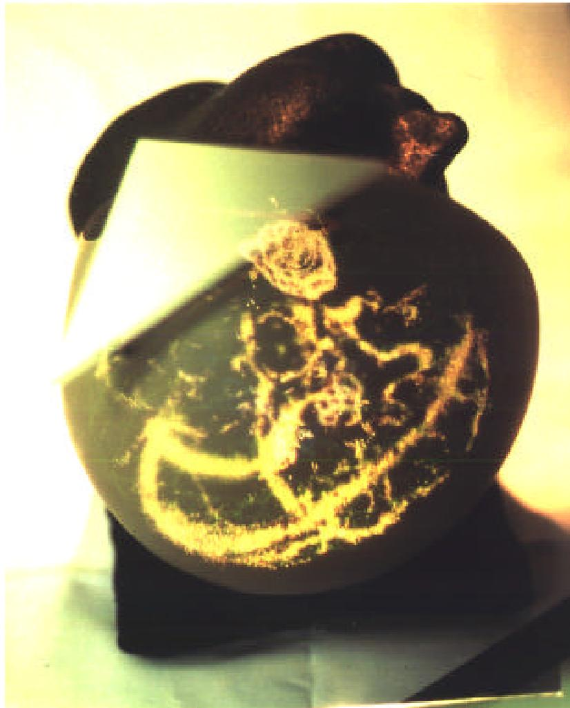
Fig. 11 Superposition of the virtualized human body over the real body(application of the augmented reality)
